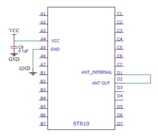
The on board high-gain antenna, if you need to use the onboard antenna, you should short the ANT\_OUT and ANT\_INTERNAL pins.
