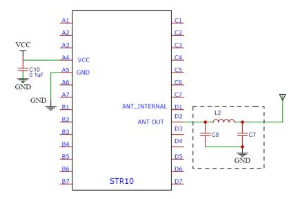
For longer distance application, use the ANT\_OUT pin to connect an external antenna. In the case, pi-network is a very flexible way to tune an antenna, which can be used to adjust the RF matching parameters .This is optional circuit, but recommended to use.
